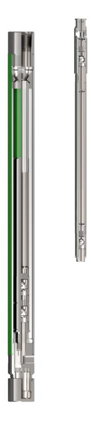
In wells with sand, grit often wears the plunger and the working surface of the pump barrel, which results in an increase in the fit clearance, a reduction in pump efficiency, and even a serious pump stuck in severe cases. In addition, for open sand content wells, ordinary pumps bury phenomenon is serious. In this regard, Weima designed and developed a long plunger sand setting pump that can be used in wells with high sand content and interstitial wells with sand content of less than 3%.
